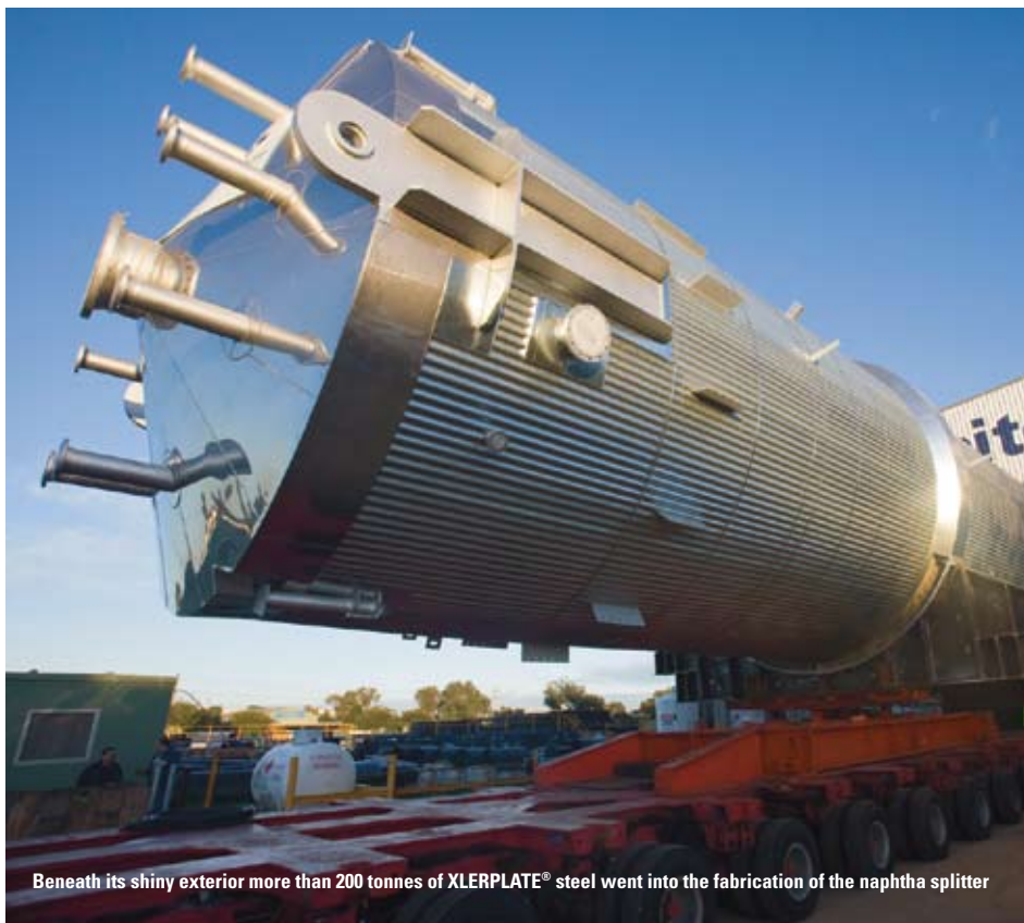
The splitter column was delivered to the BP refinery using heavy-lift specialised transporters
